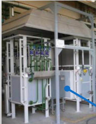
**Pressurized gasification and oxy-combustion in CFB reactor (50 kg/h)**
