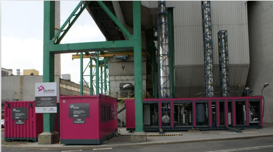
PDU for CO<sub>2</sub> capture process – 100 m<sup>3</sup>/h (2012-IChPW Zabrze)
